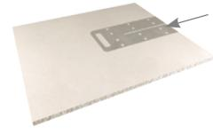
3) Run the gypsum wallboard cutter down the template to cut the slot
