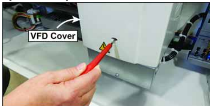
Figure 4: Inserting Screwdriver into VFD Cover
