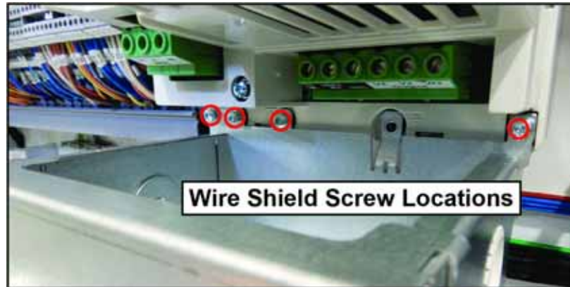
Figure 11: Wire Shield Screw Locations
