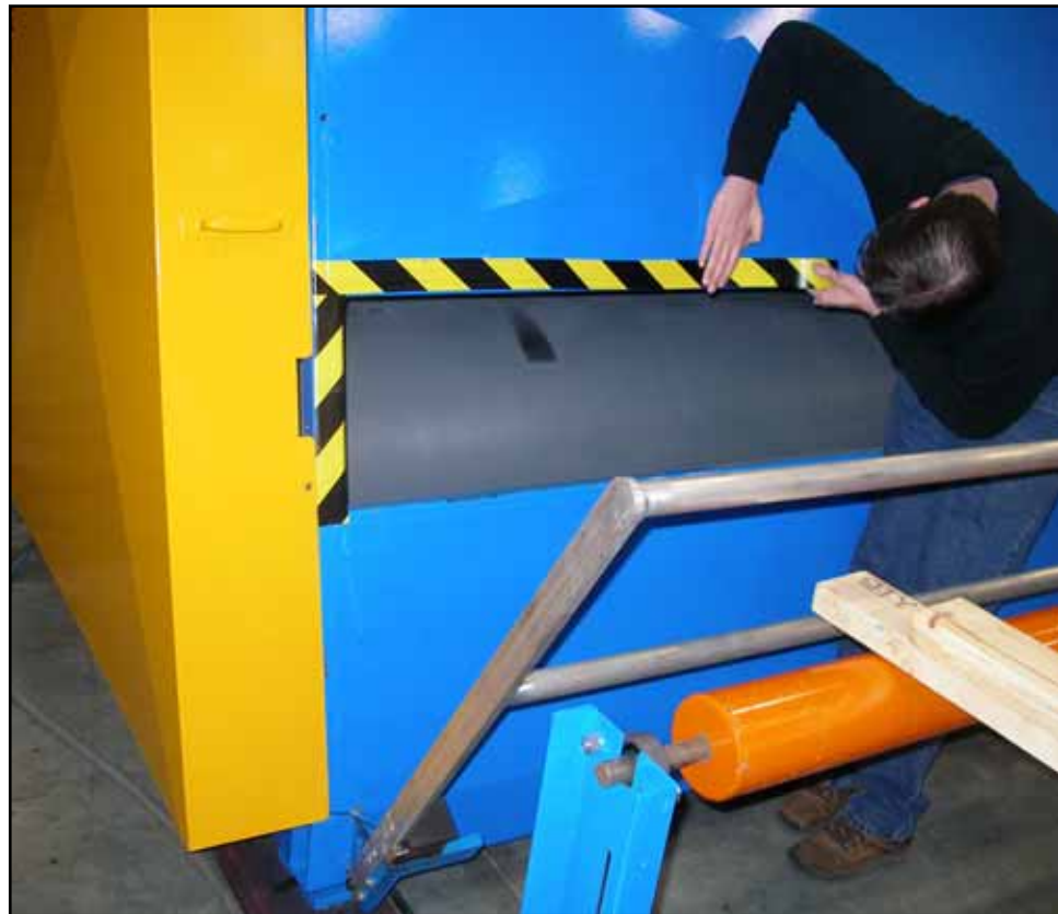
Figure 3: Applying the Warning Tape
