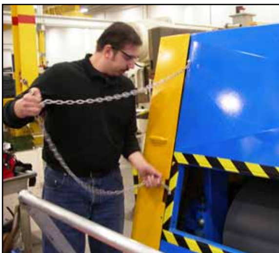
Figure 7: Attaching the Chain to the Pushbar
