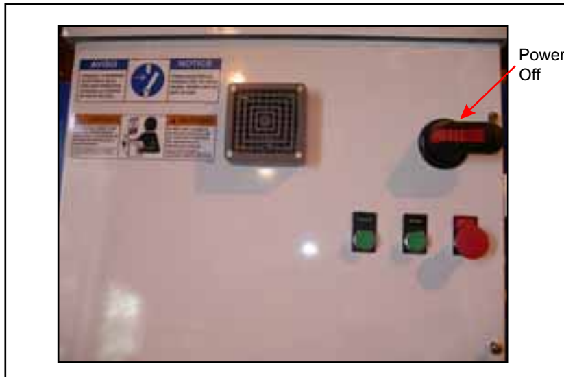
Figure 1: Power Off Switch
