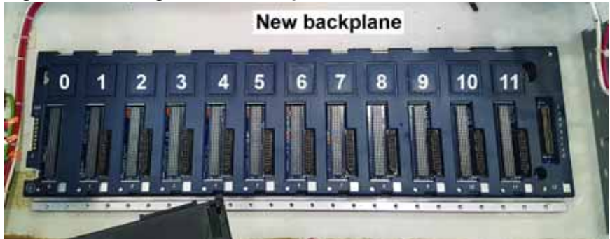
Figure 10: Placing the New Backplane
