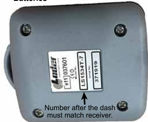
Figure 2: Remove Screws to Access Batteries
