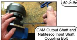
GAM Input Shaft Coupling Bolt 50 in-lbs
