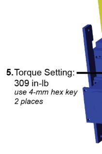
4. Tighten coupler between motor and gearbox.
