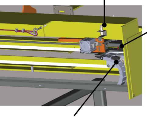
**3.** Check timing belt tension moves 1/4" up an down. Check pulley: teeth should not be worn and shaft should not have movement.
