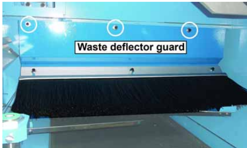
Figure 6: Installing the Waste Deflector Guard
