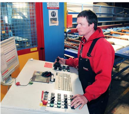
National Lumber runs automated saws guided by the SAPPHIRE BIM models, which are in turn driven by SAPPHIRE design files. As a result, National Lumber’s components and framing kits are accurate to 1/16th inch.
